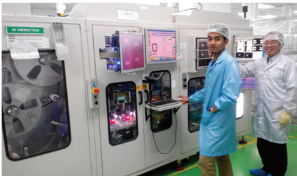
Offline Encapsulation Equipment (OLE) that dispenses and cures adhesive onto flex circuit
